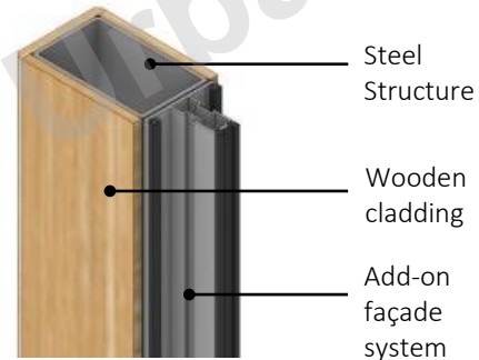
Composite Structure Steel Mullion with Wooden Cladding
